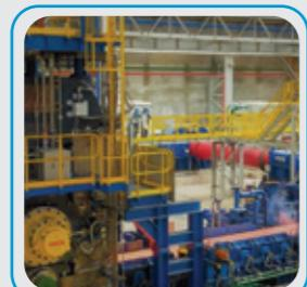
HSM has two Roughing Mill Stands and four Finishing Mill Stands. Automatic control of rolling process and process parameters
