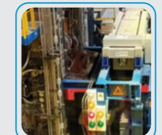
Automatic quality control with profile gauge IMS, using X-ray generator to measure parameters of thickness, width, flatness, etc. for product mix change
