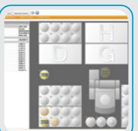
Chemical compositions are analyzed by Herzog automation system. Test results will be uploaded and stored in SAP software production management interface.
