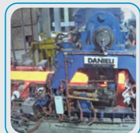
Continuous casting and rolling production line of TSC and HSM. Automatically adjust slab profile. Automatic control of process parameters
